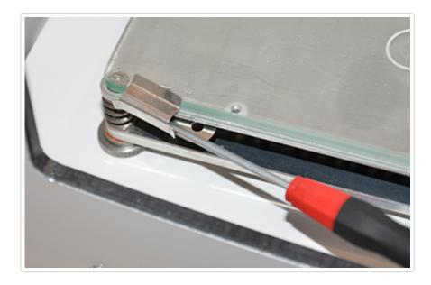
Push the glass plate into the clips in the back of the printer. Sometimes it helps to tilt the glass at a slight angle. You might need to jiggle the glass around a bit as you push it towards the back of the printer to get it to slot into the clips. Finally lock the glass in place by rotating the front clips back.
